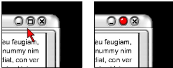
Figure 4-5 An example application of Active Cursor in a graphical user interface. Once the cursor enters the target it is dragged towards the centre of the target, resulting in easier target acquisition.
