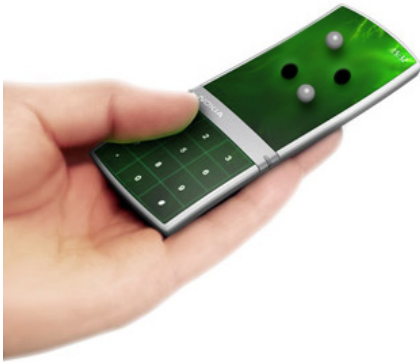
Figure 5-32: Photomontage of a digital version of the classical 'ball in the pocket' game, already described in Figure 5-30, on a tilt sensor enabled phone.
