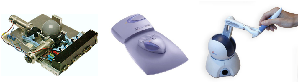
Figure 1-7 Examples of force feedback devices: from left to right: a) The IPO force feedback trackball. Not only the user, but also the system can reposition the trackball, through the two added servo motors. (Engel et al., 1994). b) The Logitech wingman force feedback mouse (Rosenberg 1996), c) The Sensable phantom a force feedback enabled 3D pointing device (Massie and Salisbury, 1994).
