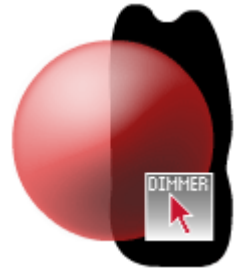
Figure 5-19 Due to the drawn ForceDimmer area overlapping the right side of the hill, only the left part of the hill will exercise force,
