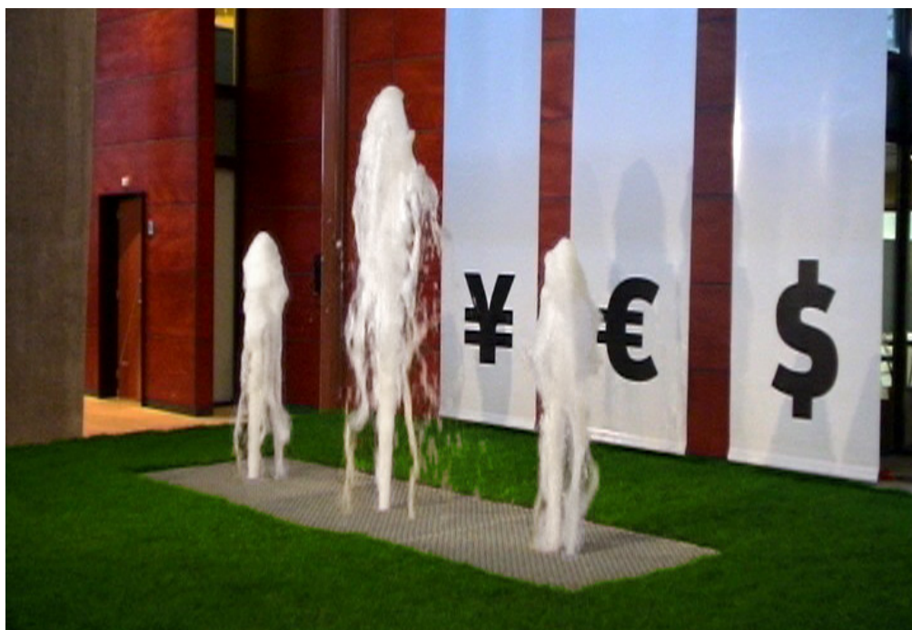
Figure 1-8 An example of digital data made physical: The datafountain translates online currency rates of Yen, Euro and Dollar to waterjets. Through an internet connection the currency rate data displayed in the water jets is refreshed every five seconds (Mensvoort 2003).
