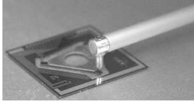
Figure 3.9: Setup used to measure the deflection of the slender rods. A triangular aluminum plate is used to create a mechanical connection between the rods.
