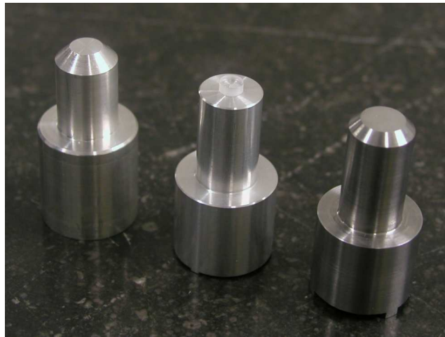
Figure 2.23: Measurement objects used in the surface force measurements. From left to right: Aluminum, sapphire and steel.
