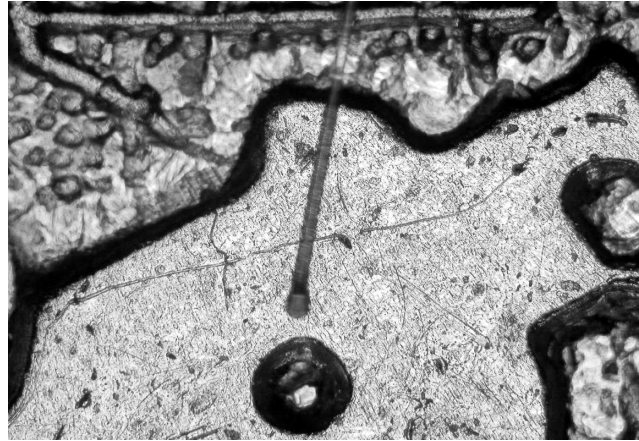
Figure 3.13: Photo of borosilicate stylus on 1 euro coin. The tip of the stylus is just above the island of Majorca.
