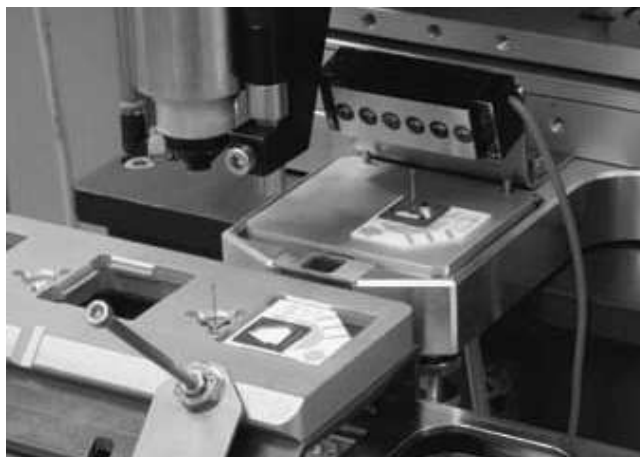
Figure 4.10: Automated assembler used to assemble the probe, photo courtesy of SenterNovem.
