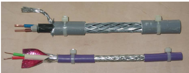
Fig. 6. Samples of (top) the armored twin lead power cable and (bottom) the shielded Profibus cable.
