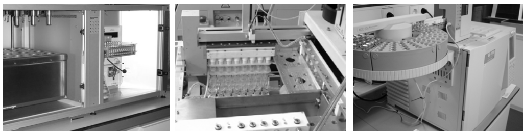
Figure 7 Pictures of the AMTEC SPR16 (left), Chemspeed ASW1000 (middle) and GC apparatus equipped with automated sampling (right)
