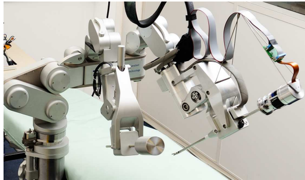
Figure 1.4 / Slave as designed and realized at the TU/e. The slave is table mounted and can be equipped with up to three instrument manipulators. (Photo: Bart van Overbeeke)
