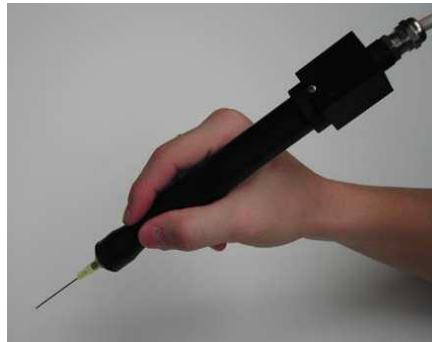
Figure 2.12 / Micron. The tooltip is actuated to compensate for tremor.
