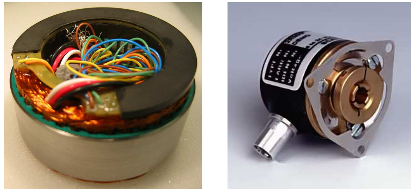
(a) frameless DC motor (stator), dimensions: \varnothing 60 \times 34 mm
