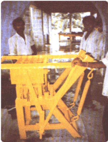
Figure 1: moulding concrete block machine (Source: Development Alternatives (2009)).
