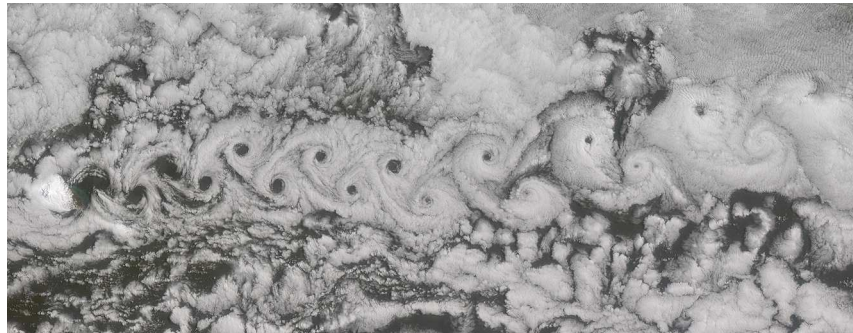
Figure 1.3 – Satellite image of the formation of a von Kármán vortex street in the wake of Jan Mayen island on June 6, 2001. The mean flow direction is from left to right and is visualised by the clouds. Image is from NASA’s Earth Observatory and spans approximately 360 by 160 km.
