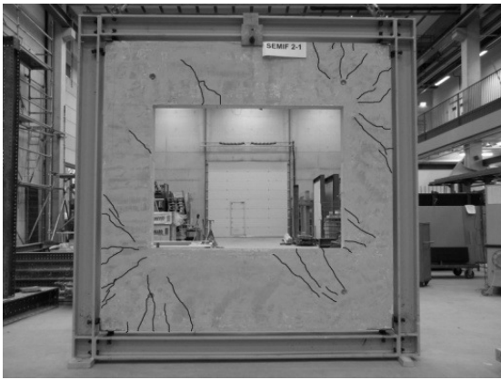
Figure C-11: Experimental and simulated final crack patterns for specimen type 2
