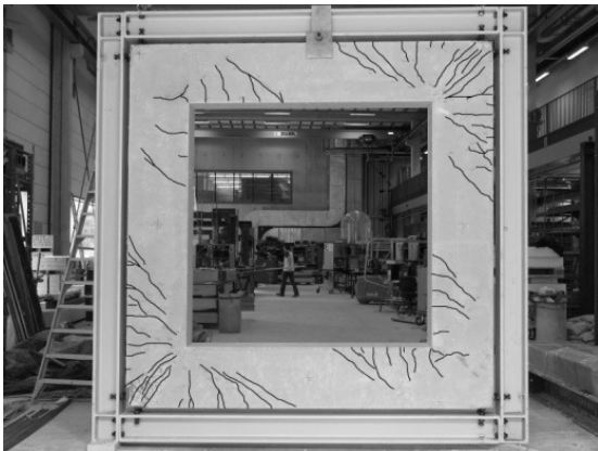
Figure C-13: Experimental and simulated final crack patterns for specimen type 5
