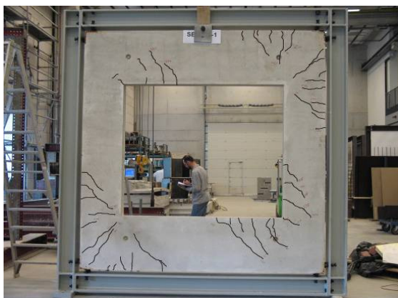
Figure 5-19: Experimental (left) and simulated (right) crack patterns (specimen type 3)
