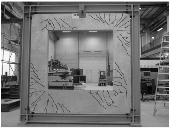
Figure C-12: Experimental and simulated final crack patterns for specimen type 4
