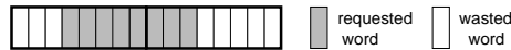
Figure 3.3: Two bursts of 8 words are required to read or write 8 words that are misaligned.
