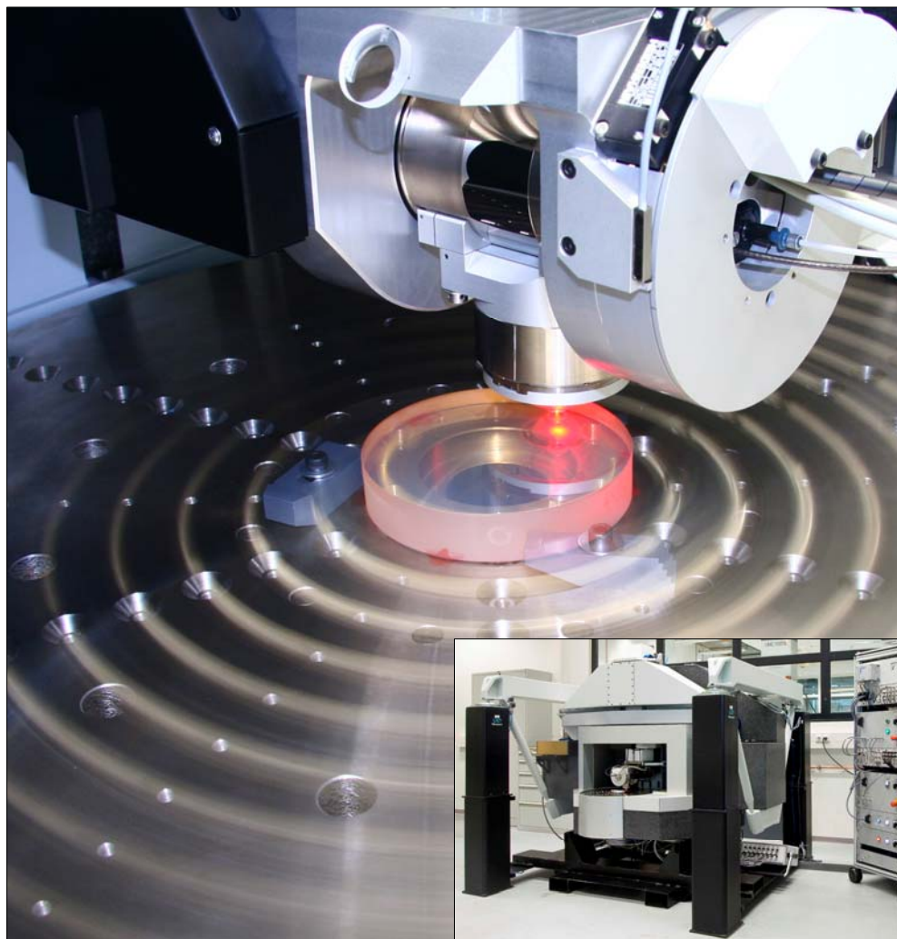
Figure 8.17: Measurement of a tilted flat (main) and the NANOMEFOS machine at the GTD workshop (insert).
