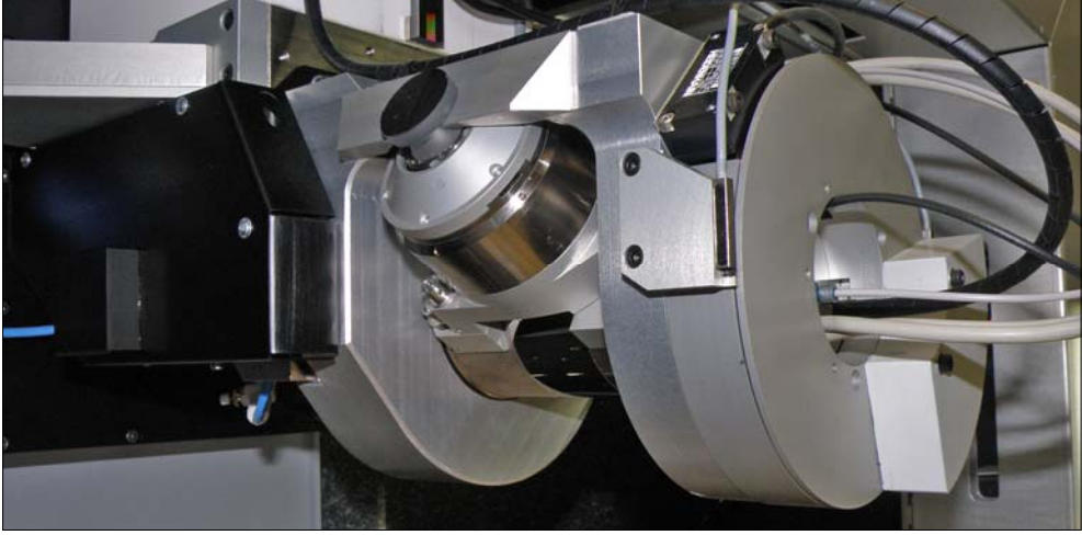
Figure 7.25: The sensor while referencing the interferometer to the reference mirror.
