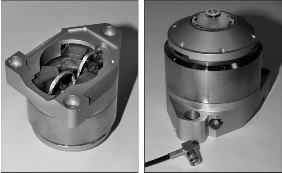
Figure 7.7: Topside of the focusing unit with the litz wires and plate springs visible (left) and the bottom of the focusing unit with the optics already in place (right), the coaxial connector can also be seen.
