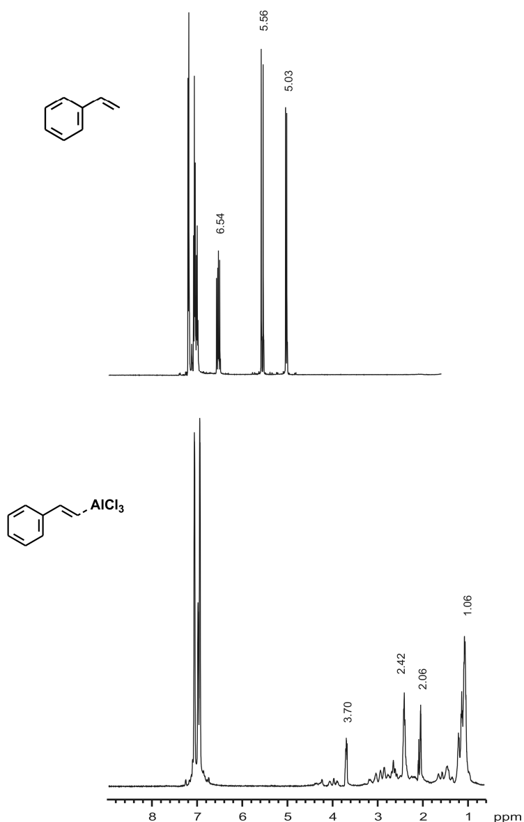
Figure 5.7. ^1\text{H} NMR spectra of styrene and styrene( \text{AlCl}_3 ) (in \text{CDCl}_3 ). The shift of the vinylic proton resonances upon addition of \text{AlCl}_3 shows Lewis acid coordination to the vinyl group.
