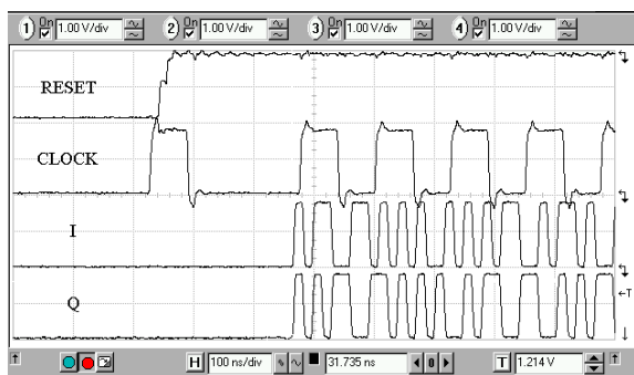
Figure 15: Gated 8 Mhz clock pulse after reset.
