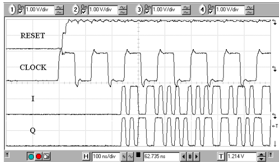
Figure 14: Non-gated 8 MHz clock pulse after reset.
