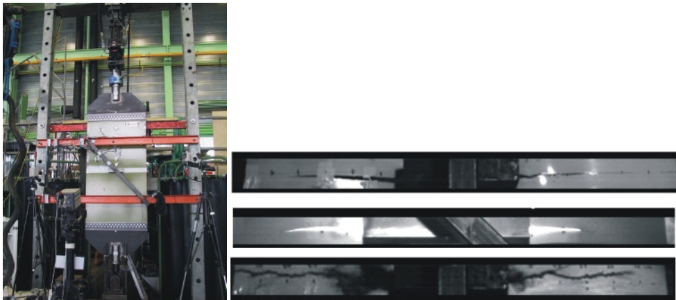
Fig. 7. (left) prestressed plate setup; (right) high speed camera snapshots during crack propagation for Aluminum (above), Glare (middle) and CFRP (below).
