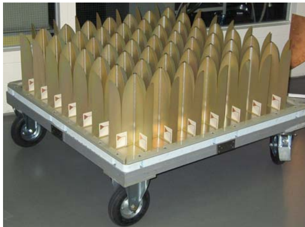
Figure 4.18: Dual-polarized array of aluminum TSA elements ( cf. ref. [23]), which is subjected to a reduced-order modeling approach.
