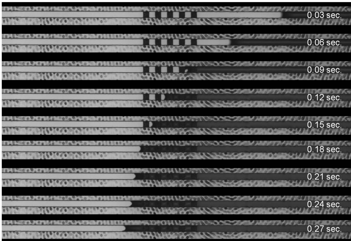
Figure 7.11: Fluid movement by capillary force through a microfluidic channel including 5 membranes.
