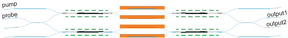
Figure 7.15: Mask design of the POLARIS all-optical switch.
