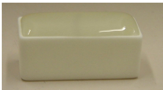
Figure 4.1: Rectangular boat used for water transpiration tests with different amounts of water in the boat. Because of different amounts of water, the height of the rim ( H_{rim} ) differs. The picture shows the boat filled with 19 gram of water. The water surface layer exceeds the height of the sidewalls by about 0.1 cm (surface tension).
