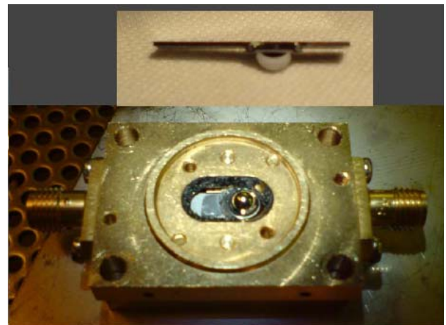
Fig. 3 The sample holder and a side view showing the synthesized elliptical lens antenna glued to the sample.
