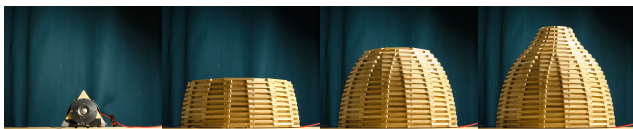
Figure 5: Scale model (1:12) of “Vox Granarium”, highlighting the tetrahedral acoustic source and 3 modular elements.
