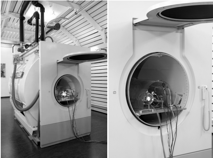
Figure 2: The magnet of the medical-imaging machine used in the spalling experiments and the experiment set-up used
