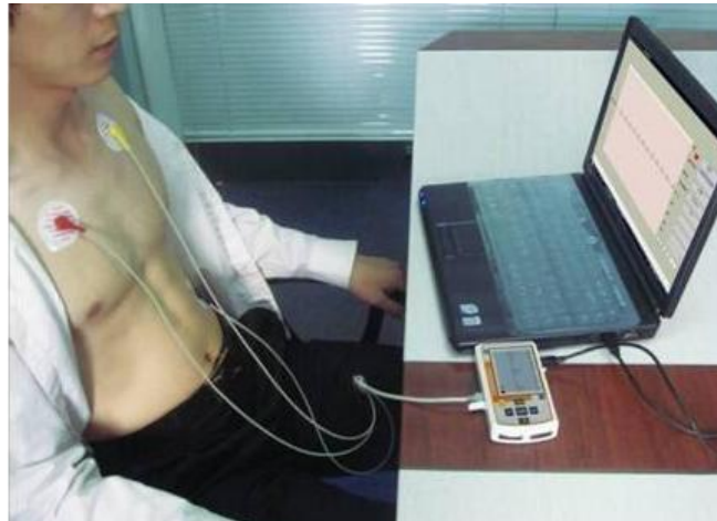
Figure 4.7: ECG monitor MD100A1 (this photo is taken from MobiKorner [125])
