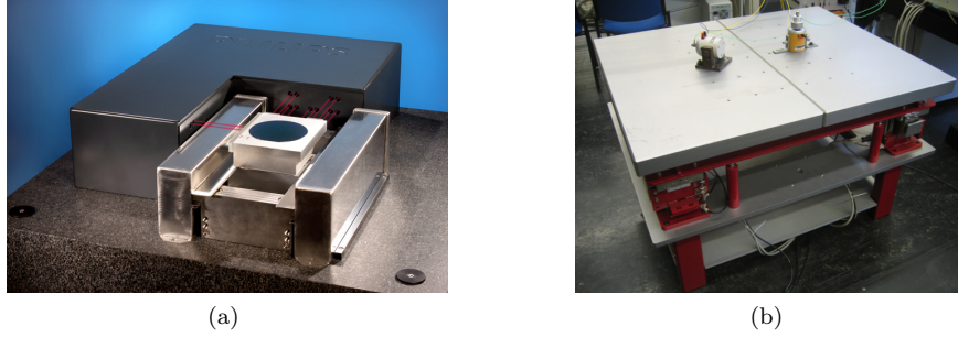
Figure 1.1: Two motion systems. Left: Multi-degree of freedom positioning stage developed by Philips Applied Technologies, [15]. Right: Active vibration isolation system developed by Integrated Dynamics Engineering.
