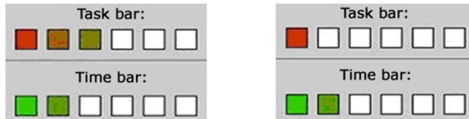
Figure 3.2: On the left: the awareness display represented Helper’s availability for communication – the task bar is ahead of the time bar meaning that the Helper advances well with the task and experiences low time-pressure. On the right: the awareness display represented Helper’s unavailability for communication – the time bar is ahead of the task bar meaning that the Helper stays behind the task and experiences high time-pressure.
