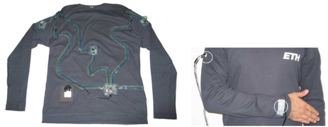
Fig. 7. (a) Inner side of the SMASH prototyping garment, including a hierarchical sensing and processing architecture. (b) Sensor positioning at the forearm and upper arm (encircled) used for model and simulation validation.
