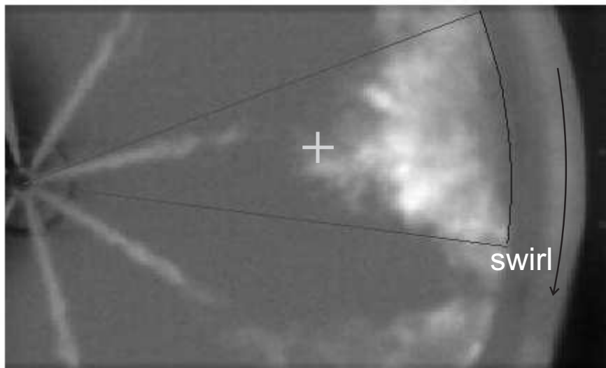
Figure 2.9: Typical CMOS camera snapshot for diesel as a fuel. The wide cone extending till the end of the field of view indicates the area where the luminosity is determined. The spray area contains scattering from liquid fuel, and is excluded from analysis. The '+' indicates the SLoL.
