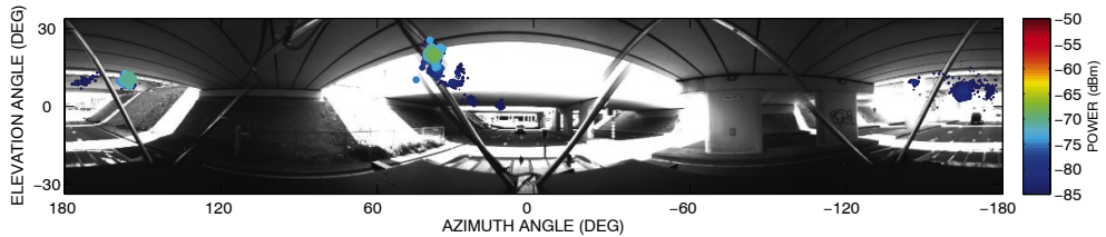
Fig. 5.11: MPC angles of arrival superimposed on omnidirectional video data for Tx at BS 7352 and k = 3100 . The received power is represented by the colour as well as the size of the markers, where the largest marker corresponds to the highest received power.
