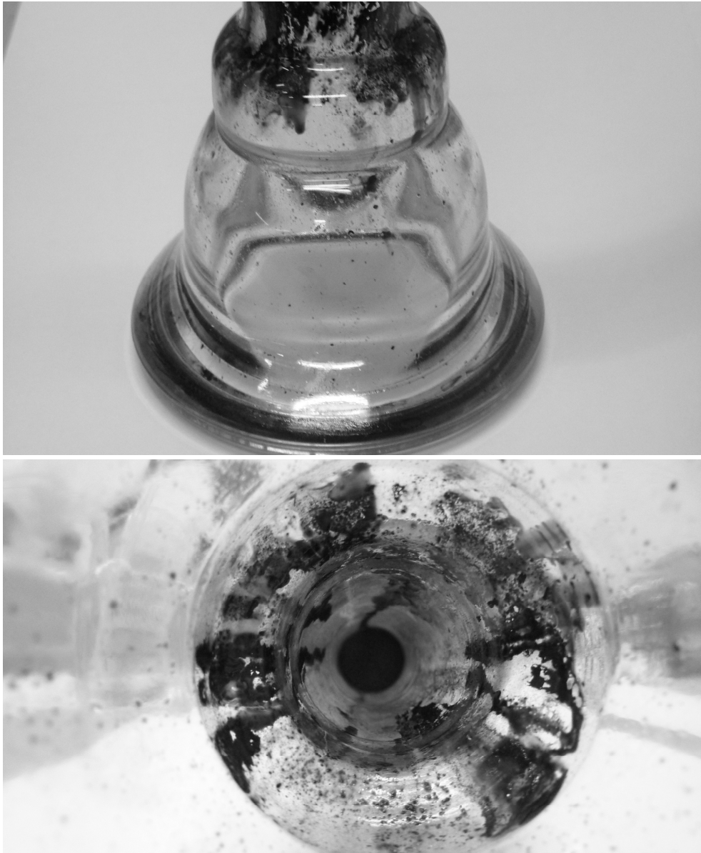
Figure 6.11: Formation of tars during biomass torrefaction in a lab scale fixed bed reactor after several experiments. The sticky tars in the reactor are shown by the black areas
