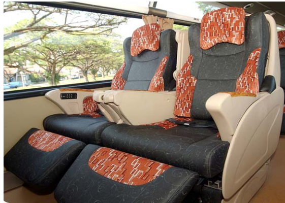
Figure 3.1 The luxury coach passenger seat with neck support (Photograph reprinted from Five Star Tours, 2010).
