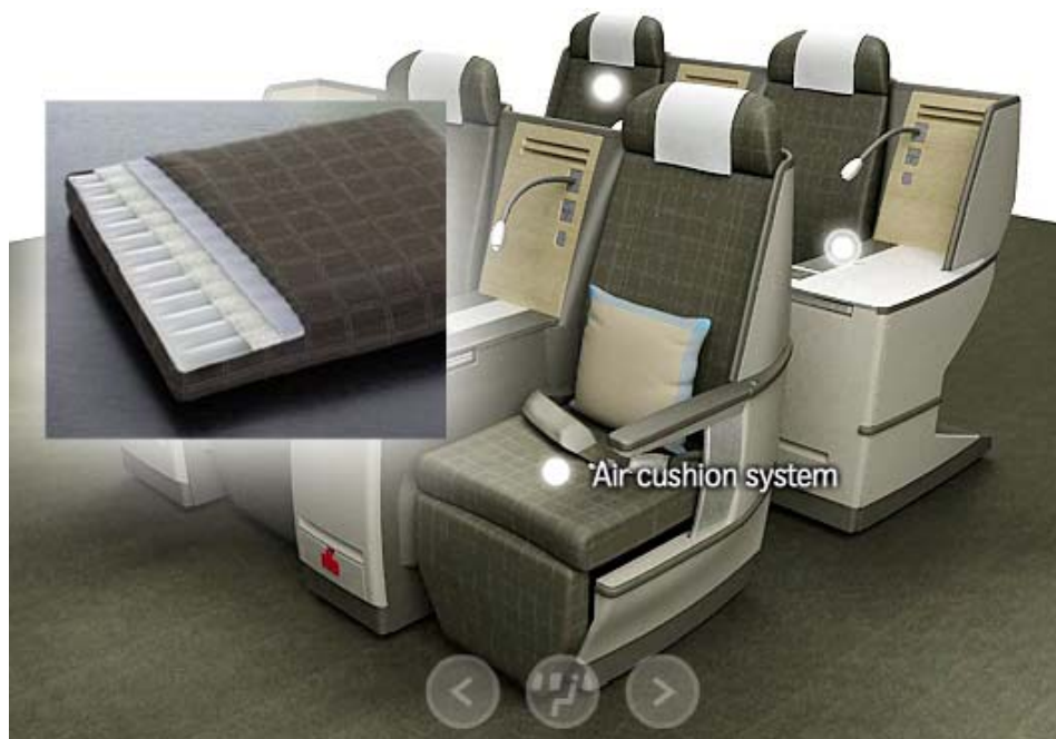
Figure 2.2 Air cushion system of Swiss Air first class and business class seat. (Photograph reprinted from Swiss Air, 2010)
