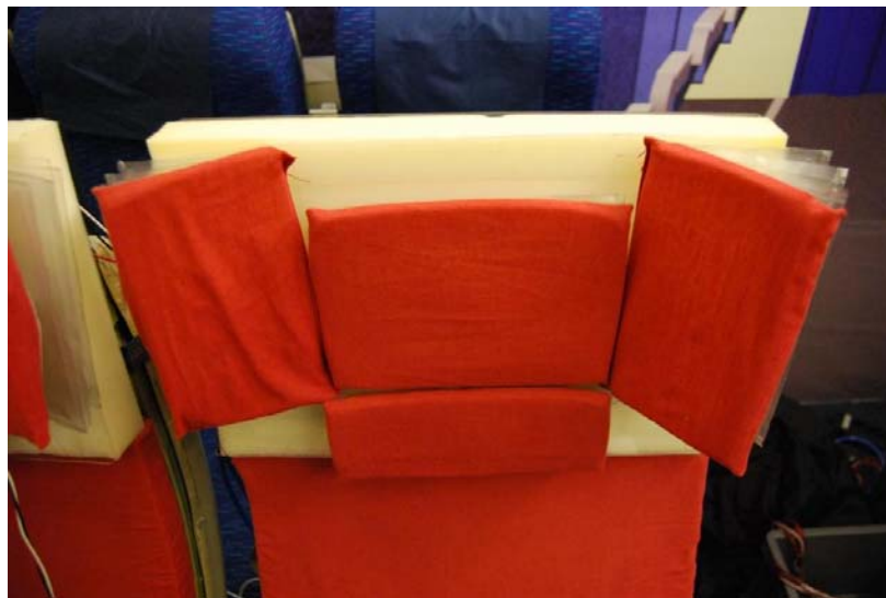
Figure 3.22 The installation of the final SnS 2 functional prototype to the economy class seat in the aircraft cabin simulator.
