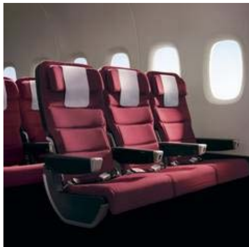
Figure 2.4 The Comfort Line 3610 economy class seat (Photograph reprinted from RECARO, 2009).
