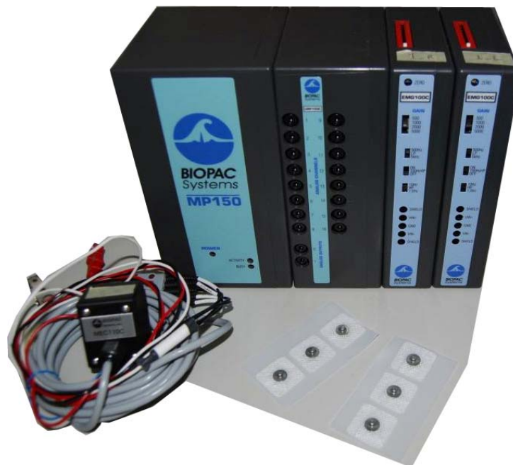
Figure 5.4 MP150 Biopac systems with electrodes and cables.
