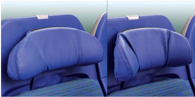
Figure 3.5 The Cathay Pacific Airlines economy class aircraft seat with built-in neck support (Photograph reprinted from Cathay Pacific, 2010).
