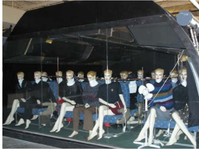
Figure 4.6 The mockup of the Boeing 767-300 aircraft cabin (Photograph reprinted from Wang et al., 2008).
