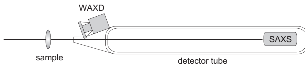
Figure A.2: A schematic representation of the experimental setup on the High Brilliance beamline ID02. 96
