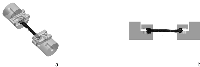
Figure 3.2: Illustration of bone fixation in the clamps of the tensile tester. (a) 3D representation. (b) Cross-section of (a).
