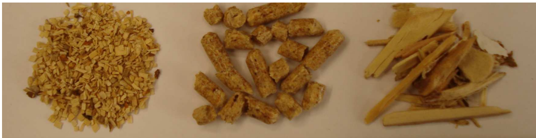
Figure 7-1: Beech wood, wood pellets and demolition wood as tested in MILENA gasifiers.
