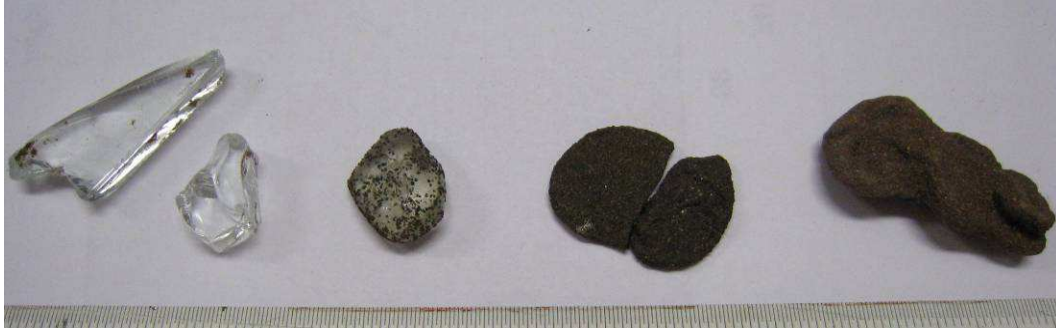
Figure 7-26: Various stages of bed material covering of glass particles.
