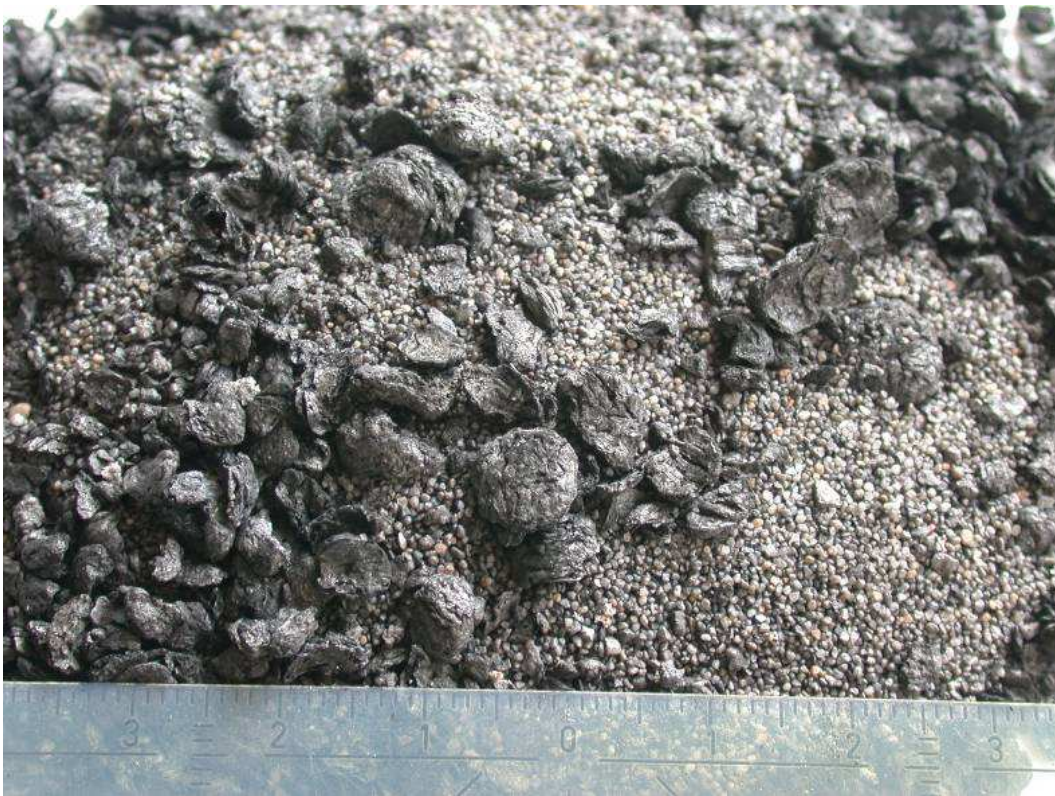
Figure 7-23: Circulating bed material from ECN CFB gasifier BIVKIN after test using wood pellets as fuel. Sand of 0.4 – 0.6 mm was used as original bed material.
