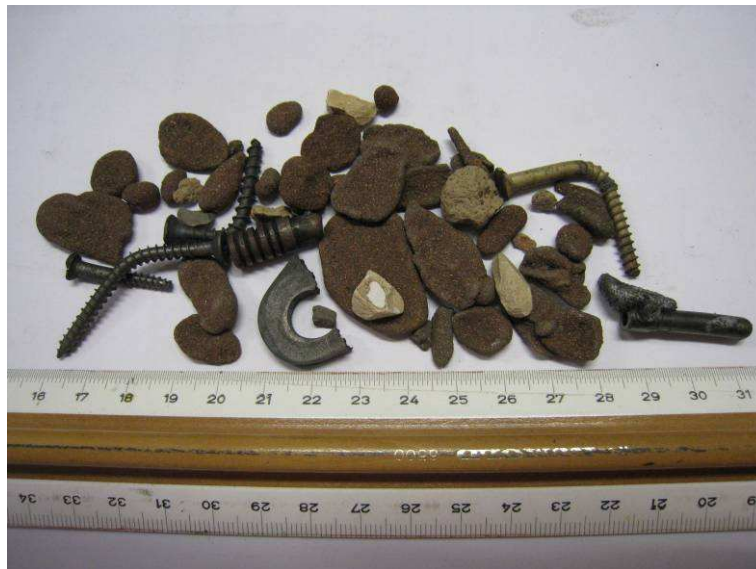
Figure 7-21: Typical example of ash particles discharged from riser.
