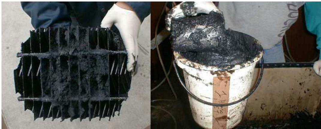
Figure 2-3: Examples of tar fouling problems
