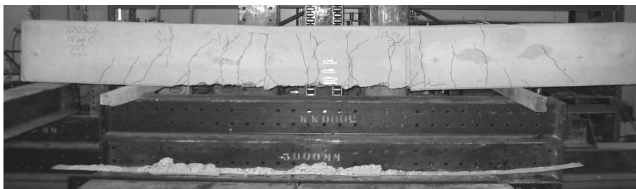
Figure 32: Large pieces of concrete remained attached to the adhesive after debonding at 70°C
