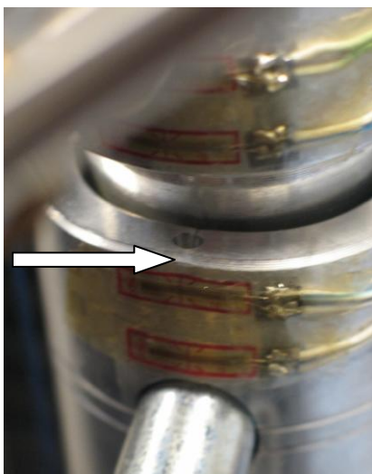
Figure 12. Start of crack at the centre point
