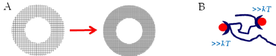
Figure 2: Encapsulation by (a) limited permeability of actives in polymer network and (b) specific binding.
