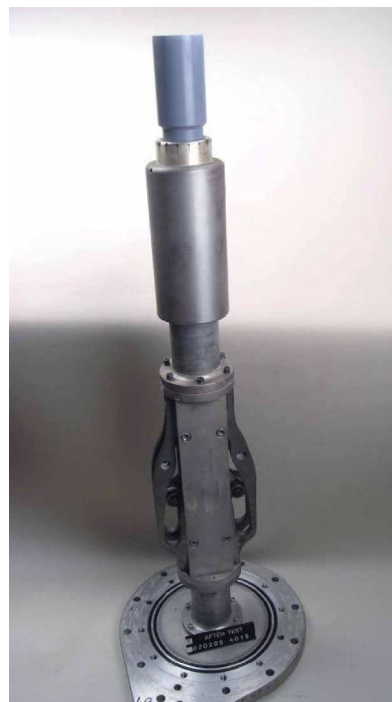
Fig. 5. Moving part of the interrupter with double-speed mechanism.
