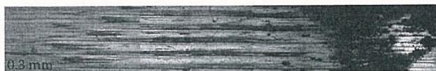
FIGURE 11.10 (See color insert.) Metal surface after the lubricity test for lubricant V551.
