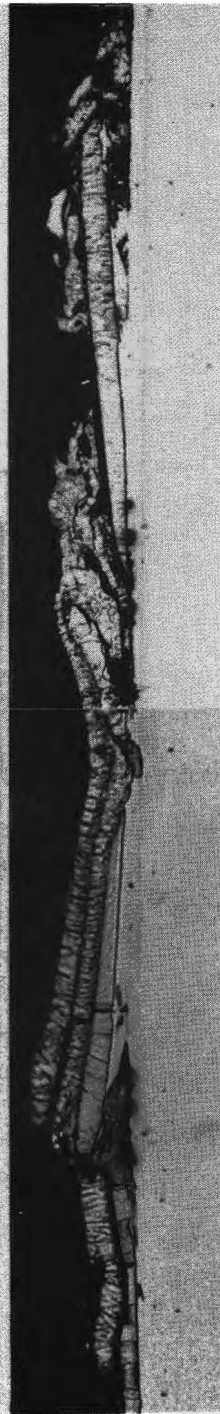
Photo 17: Cut through a free gap which has been filled up by the left particle.
