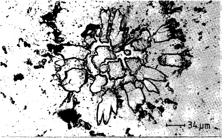
Photo 27: Flower type Mo deposit as typical for splashed super heated particles, heat content H3, experiment Mo 41.
