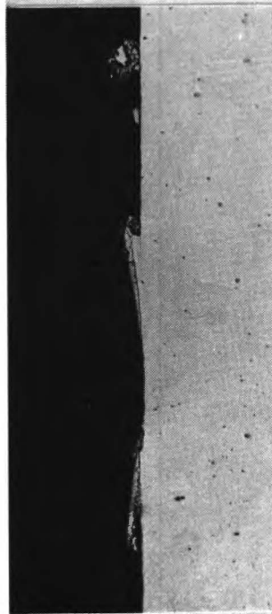
Photo 13: Cut through a flower type deposit with distinct corona on the right hand side.
