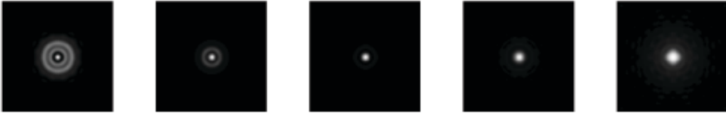
Fig. 2 Numerically computed STEM PSFs for different defocus values.
