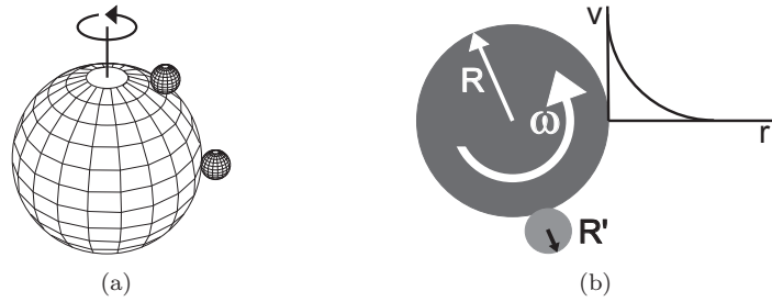
Fig. 7.6: (a) The increase in hydrodynamic drag due to the presence of a small particle attached to a large rotating particle is dependent on the position of the small particle. The hydrodynamic force on the small particle results in a torque on the large particle. The lever on which this force acts becomes smaller when the particle is positioned further away from the equatorial plane of the large particle. (b) The flow profile around an infinite long cylinder with radius R that rotates in a fluid around its long axis is given by v(r) = \frac{\omega R^2}{r} . A small cylinder with radius R' that is attached to the large cylinder experiences a drag force proportional to the effective fluid speed i.e. v_{eff} = (R + R')\omega - \frac{\omega R^2}{R + R'}
