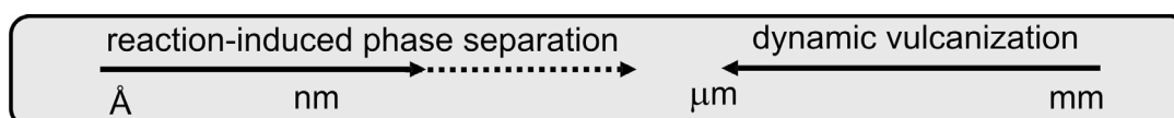
Fig. 1.7. Comparison of the morphological length scales involved during the preparation of TPVs via reaction-induced phase separation and dynamic vulcanization.
