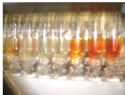
Figure 2-9: Left: Schematic representation of the synthesis of poly(styrene-block-isoprene) block copolymers via sequential anionic polymerization. Right: Image of the synthesizer during the polymerization experiment.
