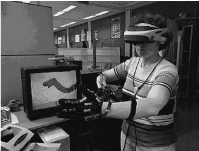
Fig. 4 MOVE ON offers the designer virtual material with which he can sketch spatially, thus intertwining the expressive wealth and 'interactive imagery' of sketching, with the spatiality and interaction possibilities of modelling.
