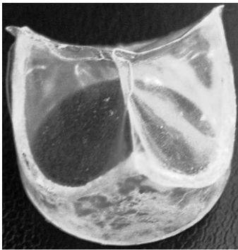
Fig. 2.5: Polyurethane heart valve leaflets fixed to a rigid polycarbonate stent.
