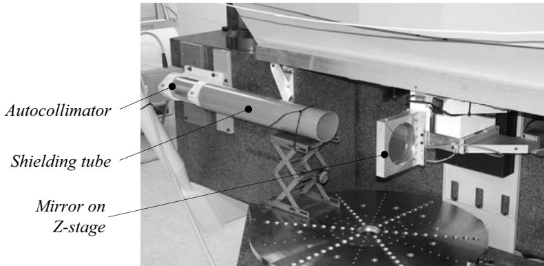
Figure 3.102: Test setup for measurement of Z-stage \psi and \theta -rotation
