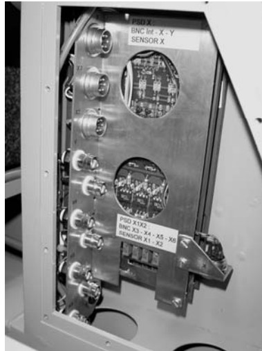
Figure 5.29: Probe electronics inside Z-stage preload frame
