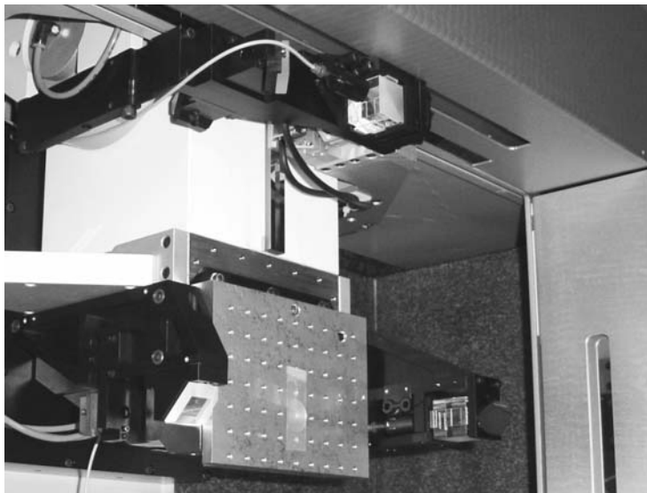
Figure 4.17: Interferometry system as assembled on the machine
