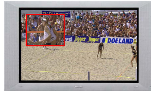
Fig. 1. The main window shows normal-play fragments with the audio also being rendered corresponding to this window, whereas the PiP window shows video corresponding to the fast search.
