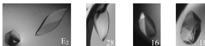
Figure 8: Co-Crystals of the ER \beta LBD in complex with cofactor peptide and the variable ligands E 2 , 28 , 16 or 18 under conditions of 0.2 M Ammonium Acetate, 0.1 M BIS-TRIS pH 5.5 and 17% PEG10000 (v/v) at 4 °C. The overall size of the crystals is 0.5 x 0.4 x 0.3 mm.
