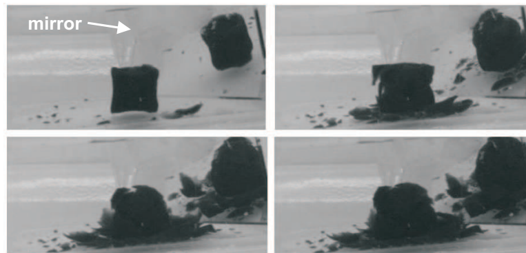
Figure 1.2: Failure of a hydrogel during swelling. Time runs from top left, top right, bottom left to bottom right.
