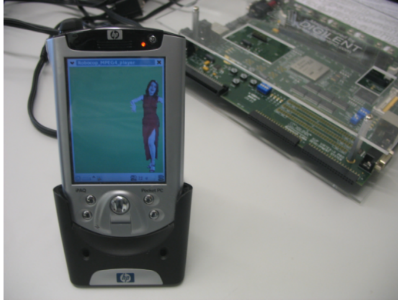
Figure 7.1: Executed MPEG-4 AS VO decoder on iPaq with ARM 400 MHz.
