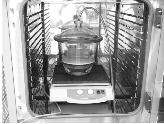
Figure 5.1: Experimental setup for groups under hypoxic conditions. The glass bell was flushed with gas mixture consisting of 7 % O 2 , 5 % CO 2 , and 88 % N 2 , and was continuously shaken to promote gas exchange and diffusion.
