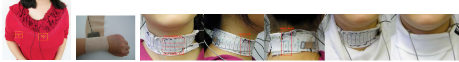
Fig. 3. Different sensor setups with which experiments were performed. Chest placement, wrist placement, and neck placements. For the neck setup, sensor placement in an elastic band and integration in a pullover collar are shown.
